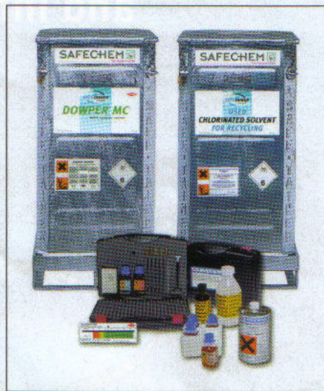
Regular checks with test kits enable the alkalinity level and the acid acceptance of a solvent to be measured quickly and accurately.
