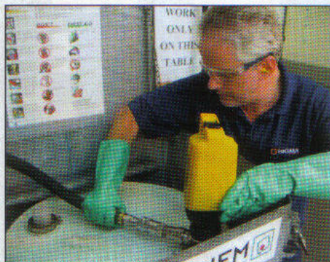
The SAFE-TAINER system comprises two separate, specially designed containers – one for fresh and one for used solvent. It is portable and integrally bundled, facilitating safe and simple on-site storage and transfer.
