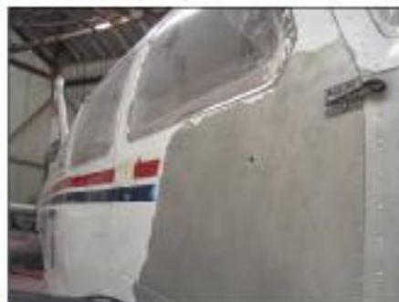
Plastic media stripping (PMS) is used widely for removing paint from civil and military aircraft.
